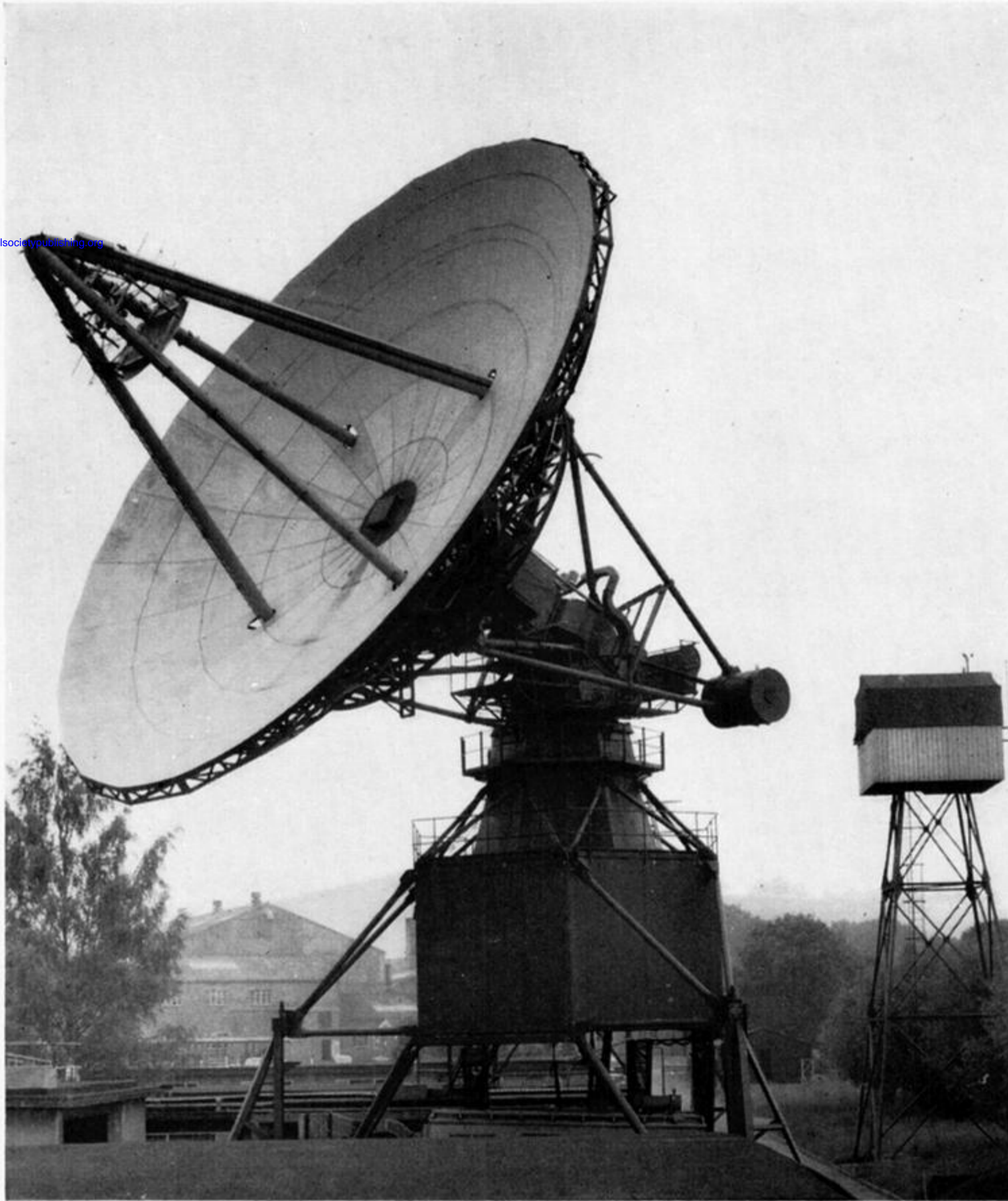
FIGURE 1. The 45 ft. diameter satellite tracking radar at the Royal Radar Establishment, Malvern. (Reproduced by permission of the Controller, H.M.S.O.)
